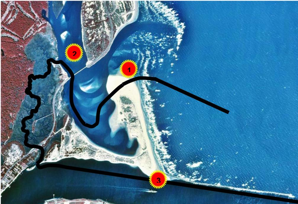
Figure 4. Three proposed borrow areas identified for the “Backpass and Bypass Sand at Ft. George and St. Johns River Entrances” potential demonstration project
