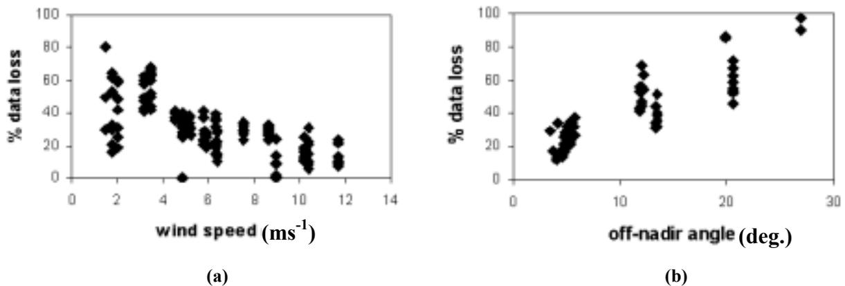
**Figure 6: Percent of data dropouts relative to a) wind speed for data collected on 9, 10, and 14 December (off-nadir angle was less than 15 deg.) and b) off-nadir angle on 13 December (wave height was less than 1 m and wind speed was  $5\text{-}10 \text{ ms}^{-1}$ ).**
