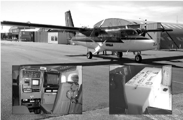
Fig. 2.3: SHOALS system mounted on a Twin Otter.
