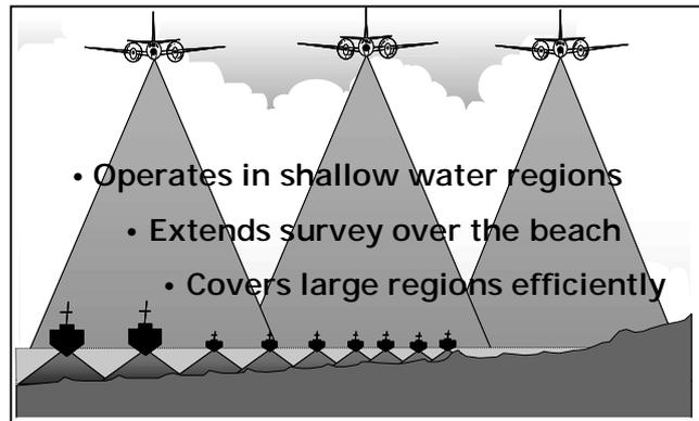
Figure 1.2: Advantage of SHOALS over multibeam acoustic surveys.
