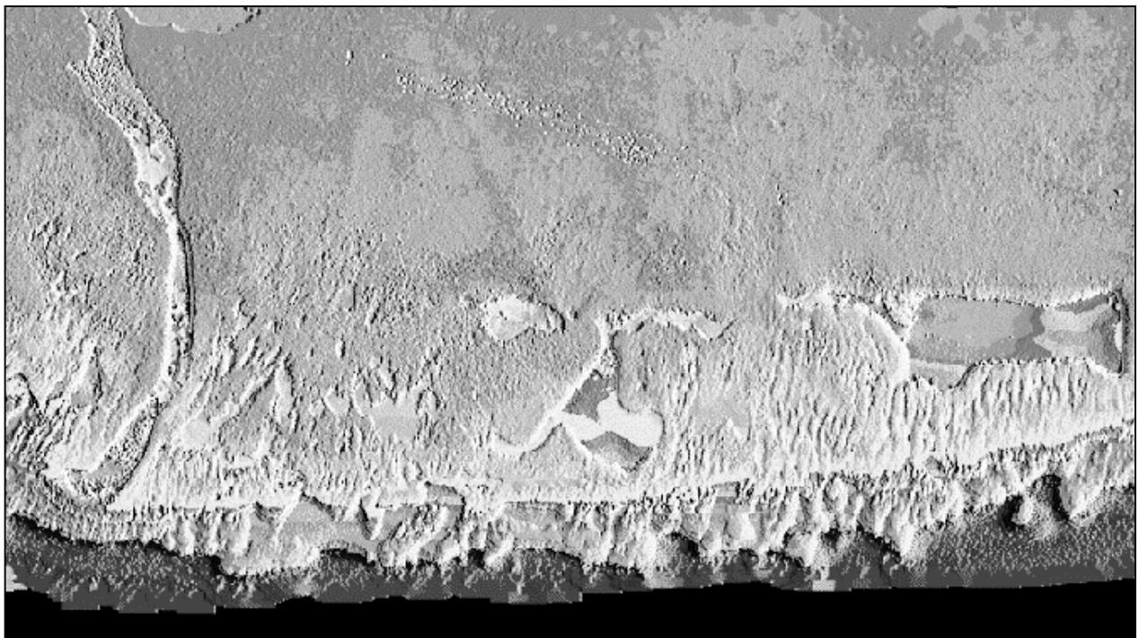
Figure 4.3: Image of SHOALS data at Molokai, Hawaii created by USGS (Wozencraft *et al.*, 2000). Shoreline is to top, offshore to bottom, and shallow to deep depths correspond with lighter to darker shading, respectively.
