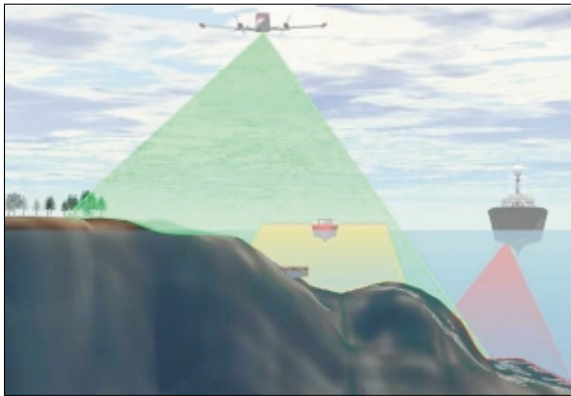
Figure 1 System Concept for Airborne Laser Bathymetry
