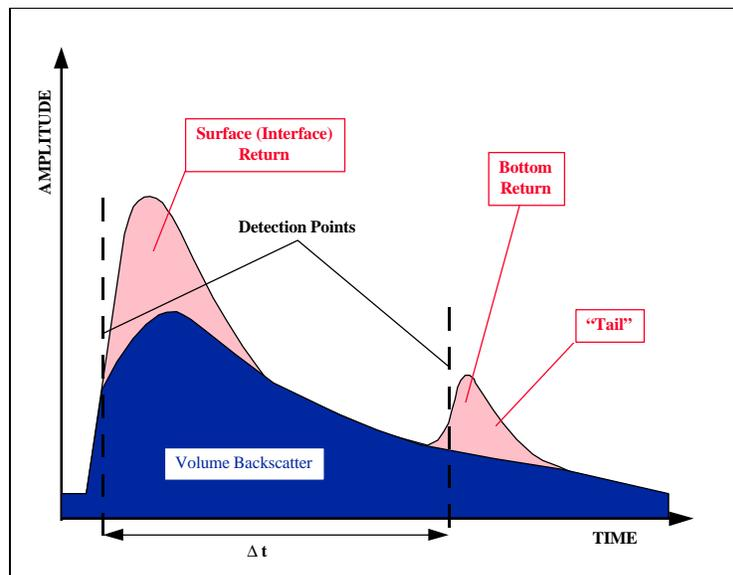
Figure 3 Generic Lidar Waveform
