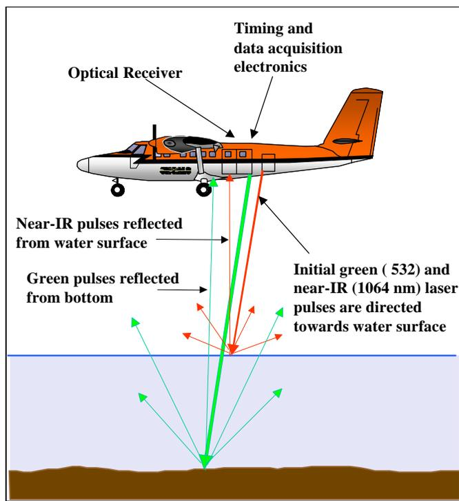
Figure 1 Principle of ALH Operation
