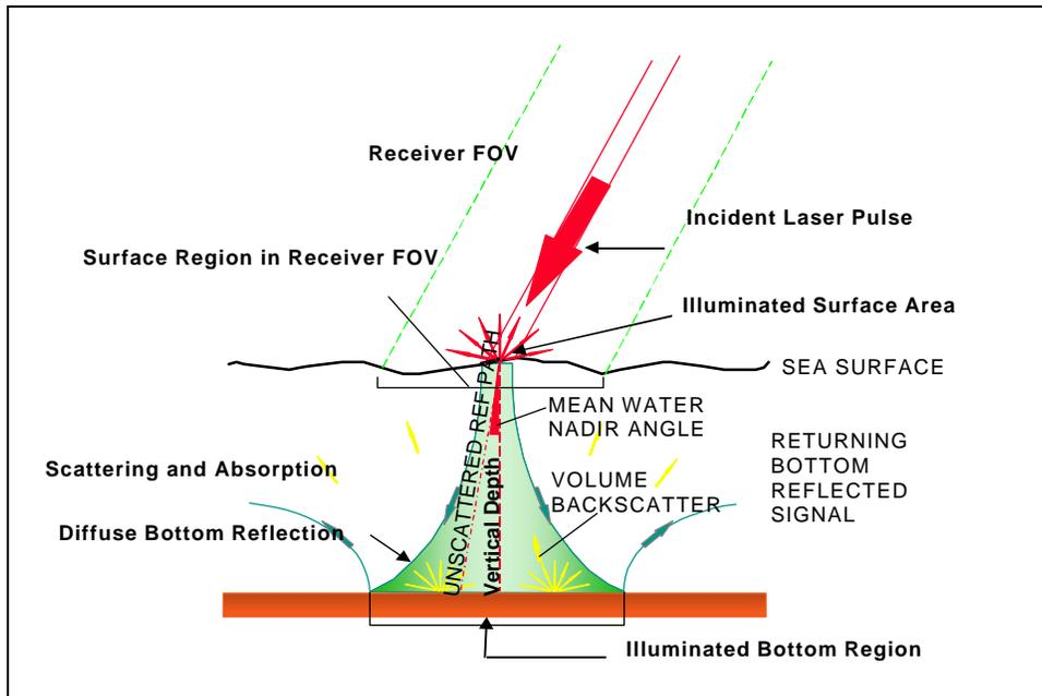
Figure 2 Geometry of Light Penetration
